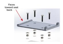
3. Align Seat Slide so the bottom slots are aligned with the holes in the bottom of the seat.
