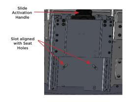
4. Attach the Seat Slide to the Seat with 1/4" bolts and washers, as shown.
