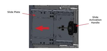
6. Align Seat Slide so the top slots are aligned with the holes in the bottom of the seat.
