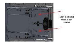
7. Attach the Seat Slide to the Seat with 1/4" bolts and washers, as shown. This is the same process as Step 6.
