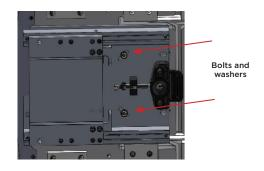
8. Activate the Seat Slide Handle and move the Slide Plate forward, as shown. Tighten the 1/4" bolts completely from Step 4.
